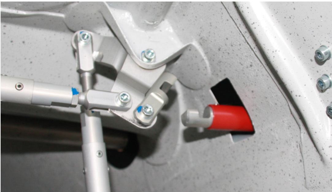
Figure 2b – opened quick- fastener
