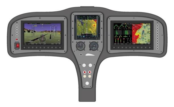
The avionics suite contains instruments from Dynon, Garmin and Air Avionics: With this extensive equipment, the REMOS GXIS is going to be certified as a LSA in Europe.
