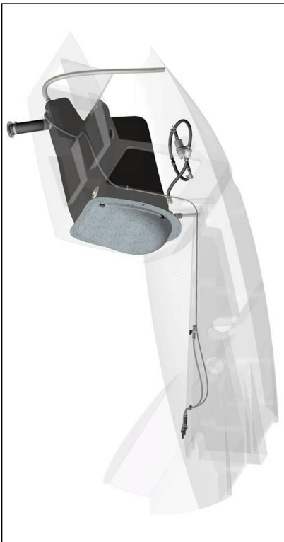
overview of airframe sided fuel system
