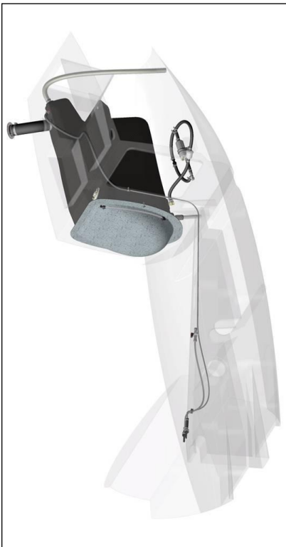
overview of airframe sided fuel system
